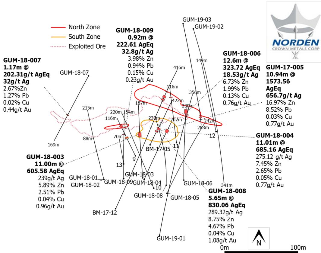
**Figure 1. Plan map showing grades for key intercepts in the main zones at Östra Silvberg.**
